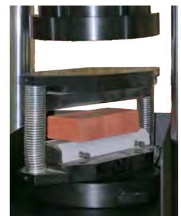
Indirect tensile of paver-bricks, as EN 1338
