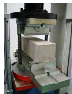
Indirect tensile of paver-bricks, as EN 1338
