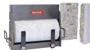
Indirect tensile (Brazilian test) as per EN 12390-6
