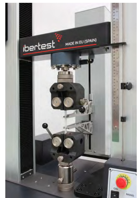
Tensile testing with a long travel extensometer. Allowing to determine elastic yield point and deformation till breaking.
