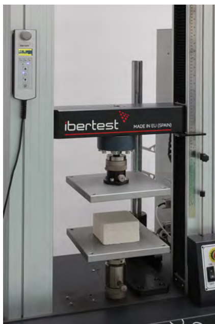
Compression test with square platens. IBERTEST supplies also circular and rectangular compression platens for fitting whatever testing requirement.
