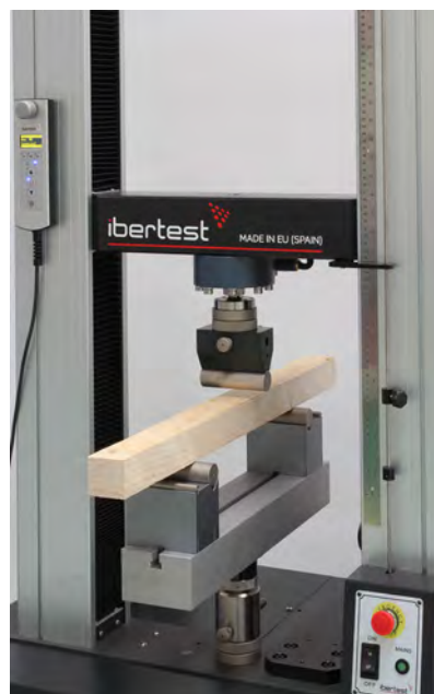
Single load bending/ flexural testing fixture. Two-points load can be applied with a double load roller bending/flexural fixture
