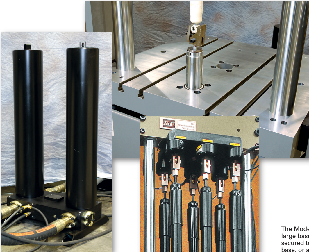
A selection of optional accumulator sizes enables you to expand Model 852 performance testing flexibility without having to add HPU capacity.
