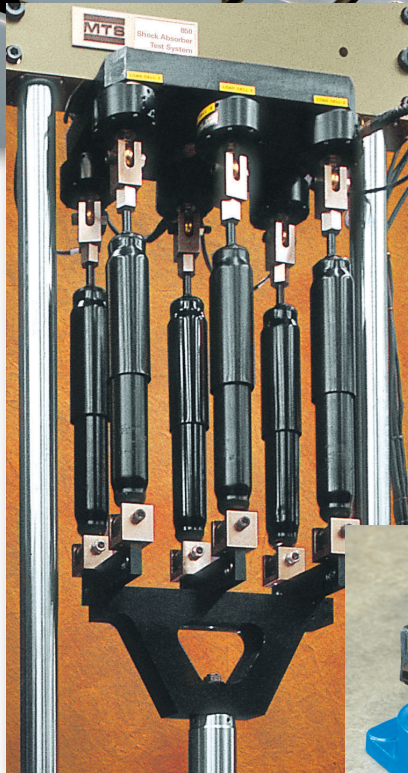
The Model 852 can perform high force and velocity durability tests on up to eight specimens simultaneously.
