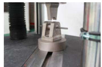
Shear testing device
