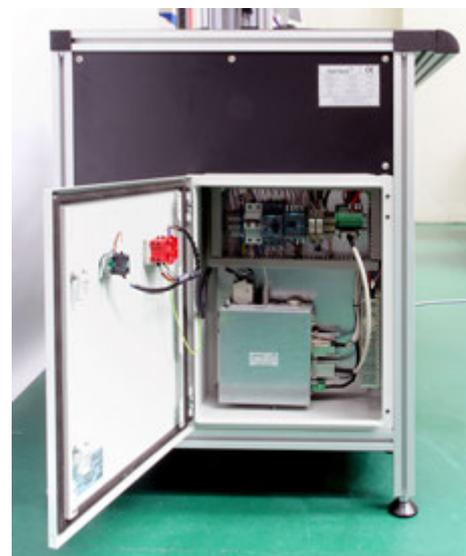
MD2i module, integrated in the electrical panel of an IBERTEST servo-hydraulic machine.
