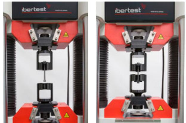
Accessory: tensile device for cabezales for button or/and threaded shoulded metallic specimens
