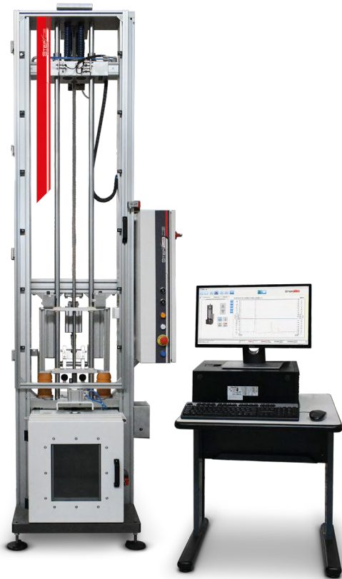
Drop Weight Tower with climatic chamber DW625
