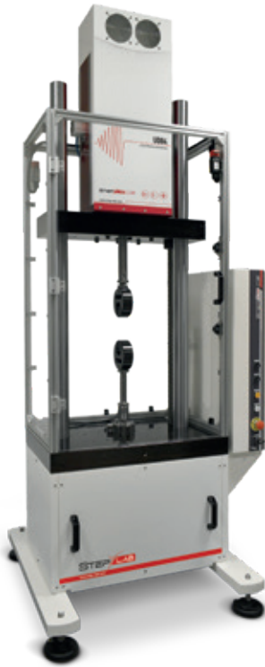
Application of the linear motor actuator UD04
