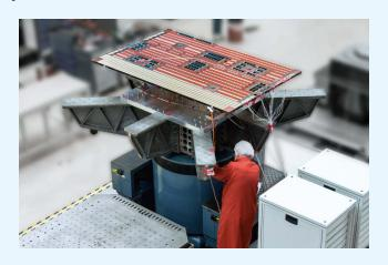
functions such as alarm and abort limits as well as notching. With force limiting, you prevent over-testing in critical frequency ranges.
